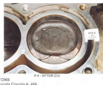
Picture I - Piston after P.i. treatment
