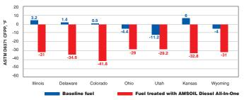
Testing reveals AMSOIL Diesel All-In-One provides significant cold-flow improvement in diesel fuels found across the U.S., delivering improved cold-weather performance.
